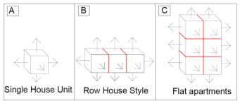
Fig (6): Surface-to-Volume (S/V) decreases from A-C with the compactness of the building shape.
