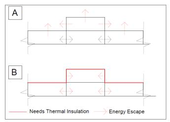
Fig (7): (A) Typical section through row houses shows energy escape due to poor insulation.
