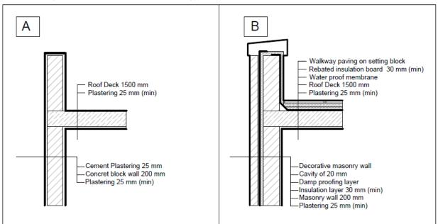
Fig (5. A): Typical roof and wall section in Kurdistan. B) Enhancement of the typical wall and roof section adding thermal insulation.
