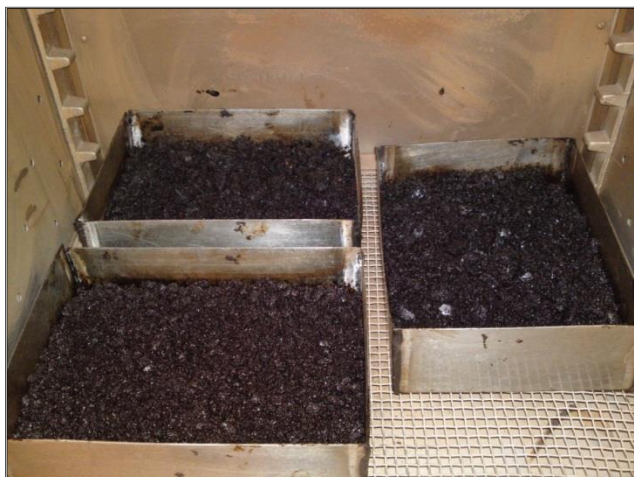
Fig (2) : loose mix in a flat pan and into a Forced Draft Oven
