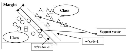
Fig 1: The Structure of SVM.
