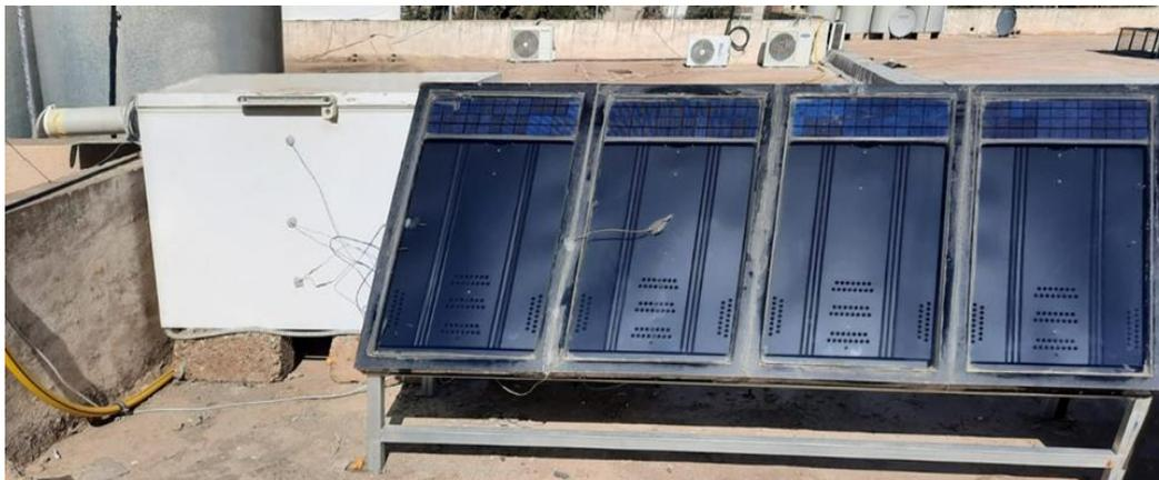
Figure. 2. A photograph of the triple-pass solar air collector with a stone storage bed
