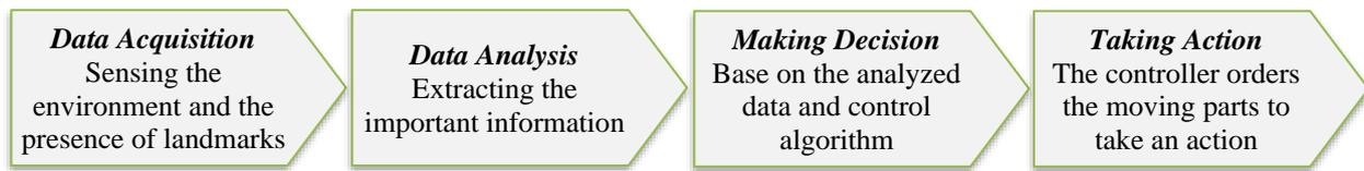
Figure (1) Block diagram of autonomous robot
