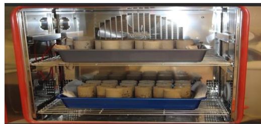
Fig (1) : Soil samples subjected to freeze-thaw cycles using a freeze-thaw cabinet
