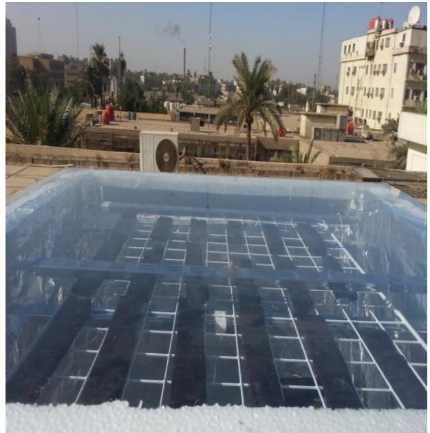
Fig (3) PCMs pieces arranged in a net under the glass
