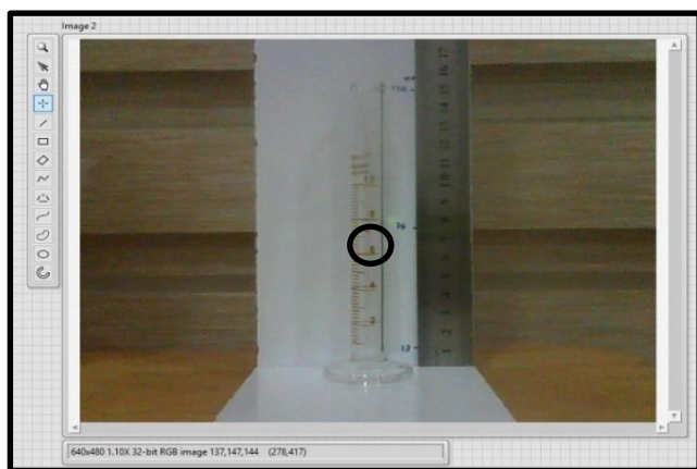
Fig (3) : Camera alignment with respect to the cylinder
