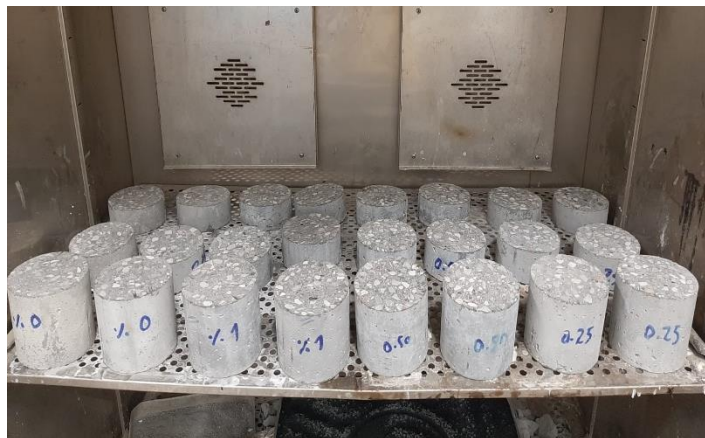
Fig. 3: Sorptivity test SCC samples
