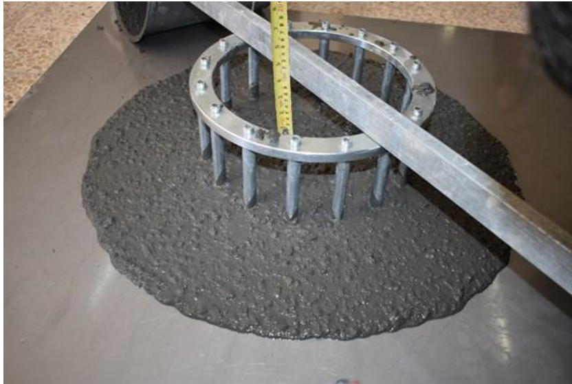
Fig. 2: J-ring test of present SCC
