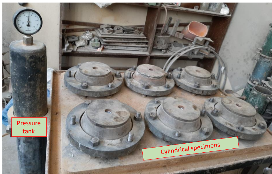
Fig. 5: Water penetration depth test set-up
