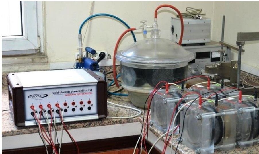
Fig. 6: Rapid chloride permeability test set-up
